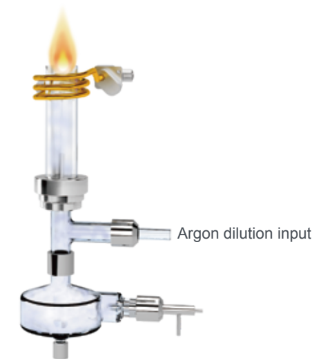
Schematic diagram for argon dilution input
