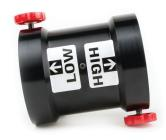
**Cal Check Standard** Used to verify sensor stability over time and transfer calibrations between sensors.
