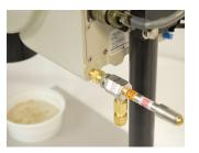
**Air Cooling** An air vortex cooler attached to the sensor for elevated ambient temperatures.
