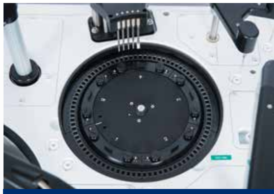
Long-life direct read cuvettes with integrated Cuvette Quality Assurance System
